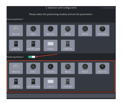
(3) Select "C-RTK 9Ps" for Positioning Module 1 and "C-RTK 9Ps UART4" for Positioning Module 2, and then fill in the antenna installation position on the right side.
