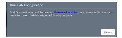
Please make sure that the positioning module is not connected to the intelligent controller, if it is connected, please unplug it immediately. Then, click the "Reboot" button. Then wait for the Intelligent Controller to reboot.
