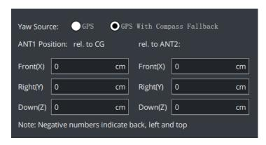
② If other products and the mounting position is not in the center of gravity, then toggle the
