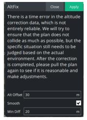
The Altitude Offset is the amount by which the known altitude data should be shifted upwards to prevent the altitudes from being too close together and causing problems;
