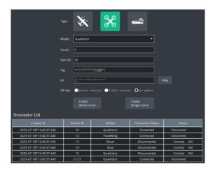
The default count of emulator is 1, only one simulator is generated at a time. If you need to generate more than one simulator at the same time, the generated simulators will be arranged in the vicinity of the specified location in accordance with specific rules, and at the same time, according to your actual need, you can choose to "Creat(Multi Conn)" or "Creat(Single Conn)".
