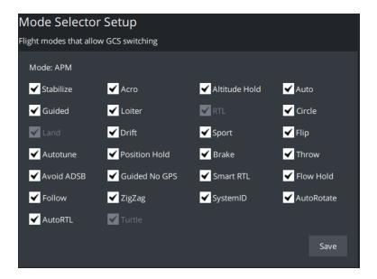
(2) Check the desired flight mode and click "Save" to complete the setting. When the storage mode is APM, the data will be written to the FLTMODE\_GCSBLOCK parameter of the flight controller; Local mode will be saved locally.
