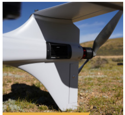
Rear Cooling Air Duct
